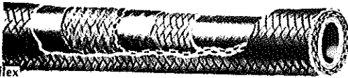
Stratoflex MIL-H-8794 hose has one steel braid and an outer cover of rough cotton braid.
