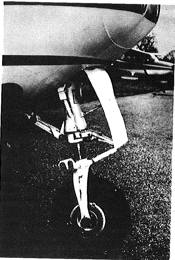
The oleo strut piston is prevented turning in its cylinder by torsion links which allow in and out movement, but no rotation.
