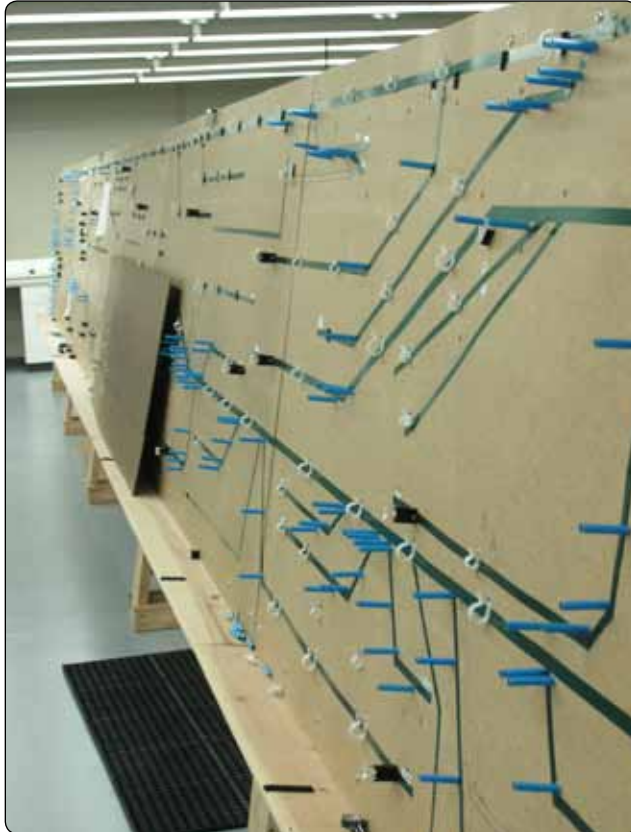
Figure 9-129. Cable harness jig board.
