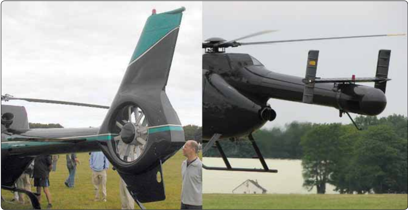
Figure 2-28. Aerospatiale Fenestron tail rotor system (left) and the McDonnell Douglas NOTAR® System (right).
