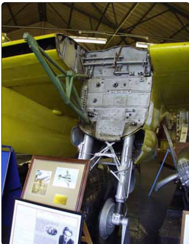
Figure 1-41. An engine nacelle firewall.
