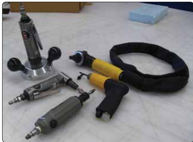
Figure 7-32. Air tools used for composite repair.
