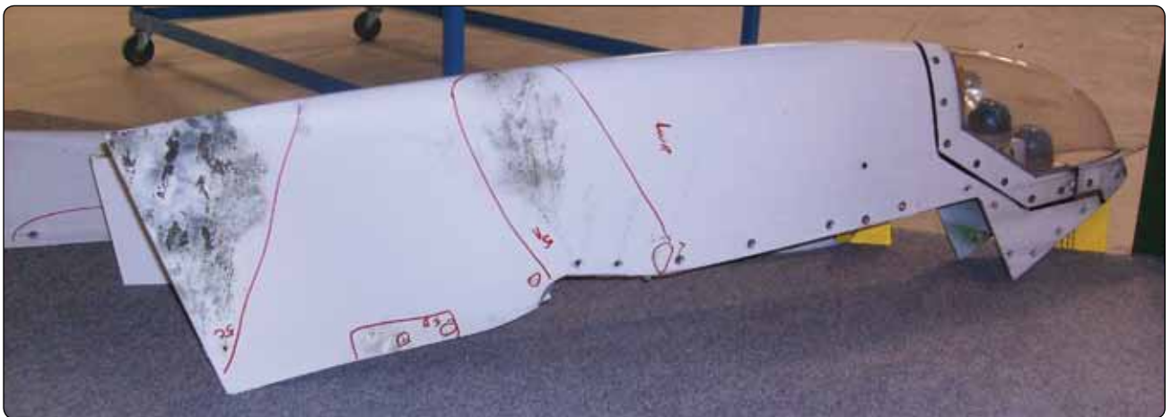
Figure 7-22. Erosion damage to wingtip.
