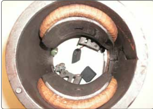
Figure 9-46. Generator field frame.
