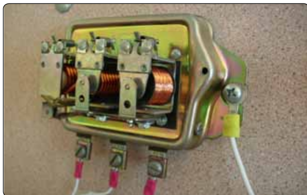
Figure 9-59. The three relays found on this regulator are used to regulate voltage, limit current, and prevent reverse current flow.
