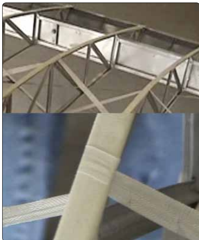
Figure 3-19. Inter-rib bracing holds the ribs in place during the re-covering process.
