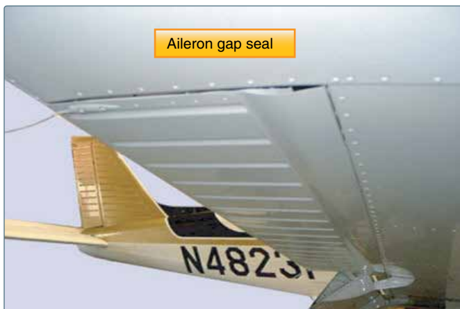
Figure 1-81. Gap seals promote the smooth flow of air over gaps between fixed and movable surfaces.
