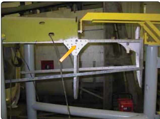
Figure 1-18. Gussets are used to increase strength.
