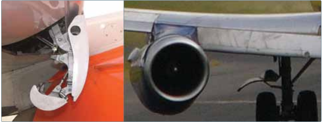
Figure 1-66. Side view (left) and front view (right) of a Krueger flap on a Boeing 737.
