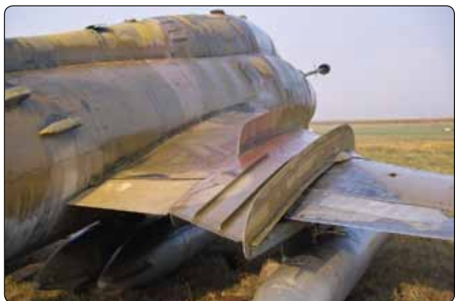
Figure 2-20. Aircraft stall fence.
