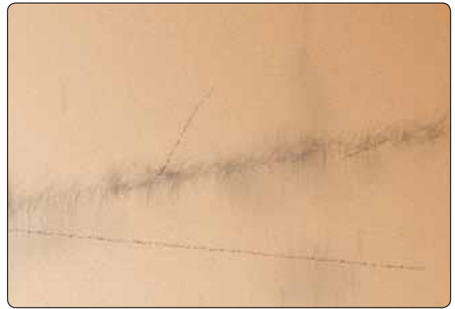
Figure 8-19. Example of sanding scratches.
