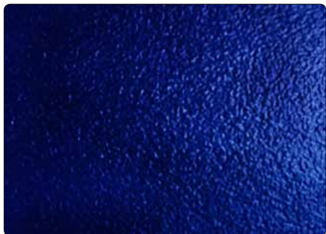
Figure 8-17. Example of orange peel.
