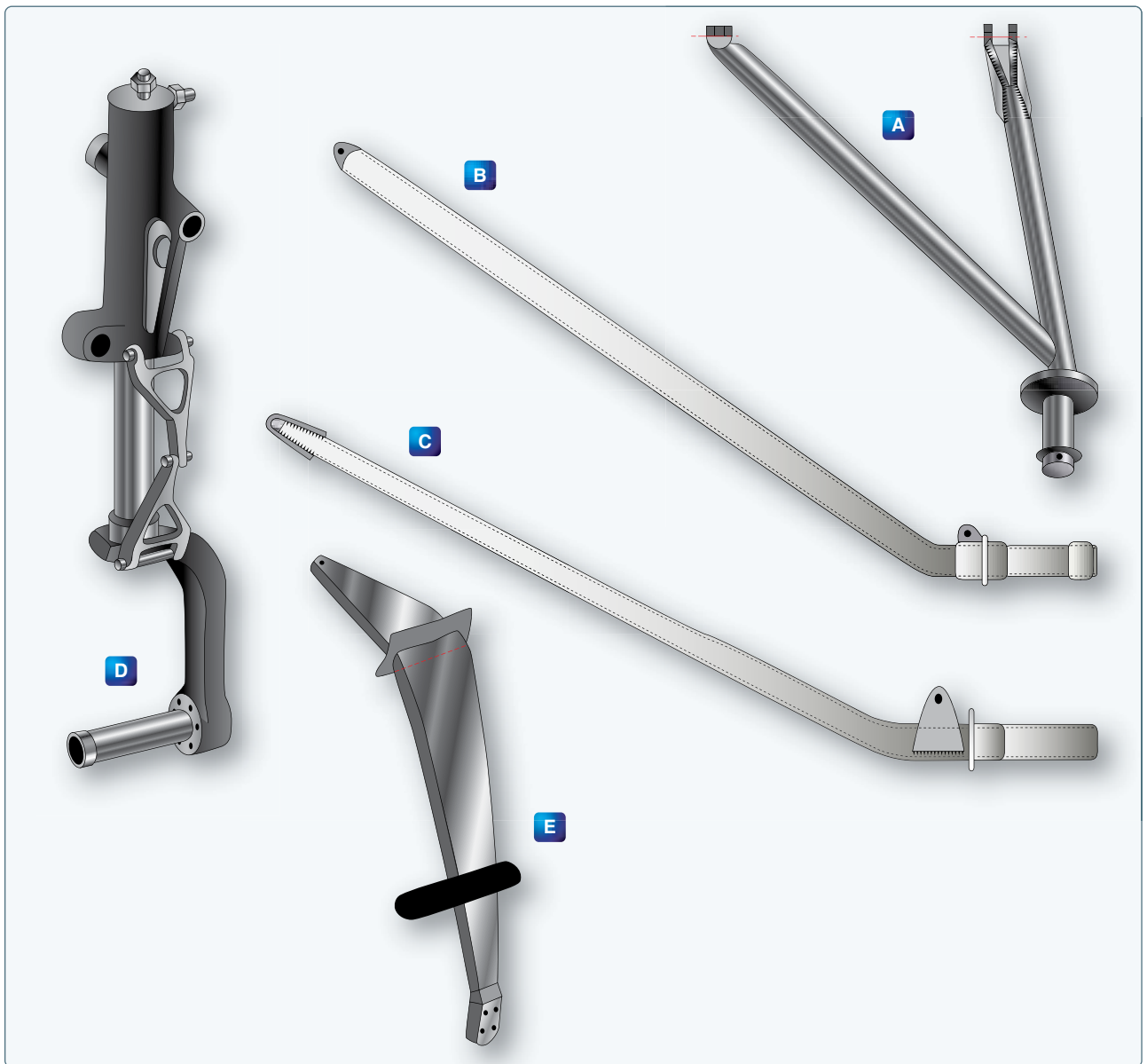
Figure 5-51. Representative types of repairable and nonrepairable landing gear assemblies.
