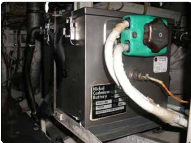
Figure 9-34. NiCd battery installation.
