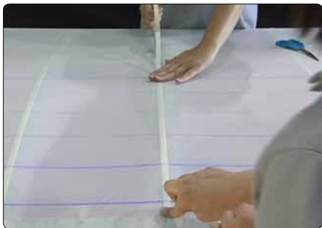
Figure 3-23. Reinforcing tape the same width as the wing ribs is applied over all wing ribs.
