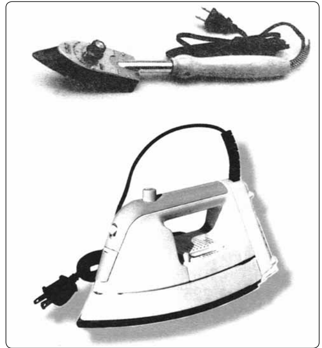
Figure 3-21. Irons used during the fabric covering process.
