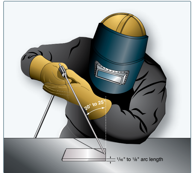
Figure 5-32. Angle of electrode.
