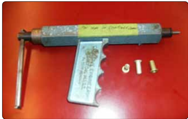
Figure 4-114. Rivet nut installation.
