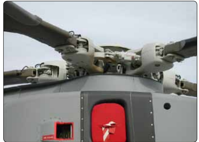
Figure 1-99. Five-blade articulated main rotor with elastomeric bearings.
