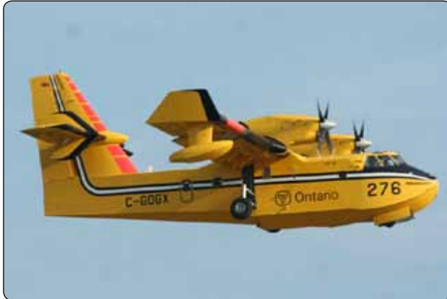
Figure 1-84. An amphibious aircraft is sometimes called a flying boat because the fuselage doubles as a hull.
