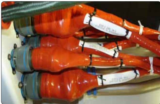
Figure 9-114. Wire harness with protective jacket.
