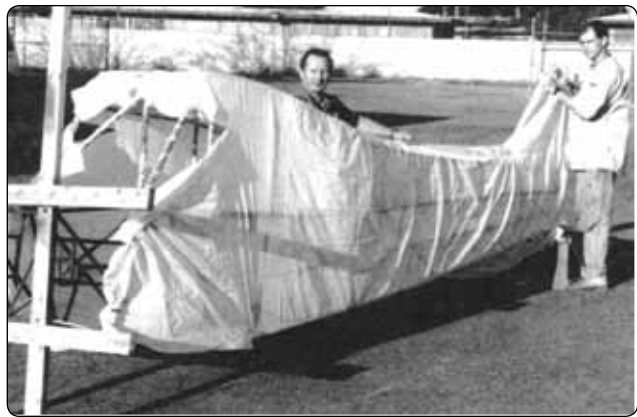
Figure 3-13. A custom-fit pre-sewn fabric envelope is slid into position over a fuselage for the envelope method of fabric covering. Other than fitting, most steps in the covering process are the same as with the blanket covering method.
