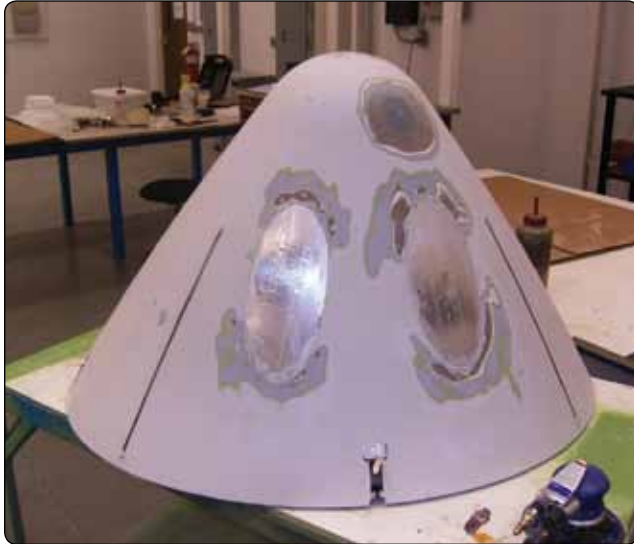
Figure 7-21. Damage to radome honeycomb sandwich structure.
