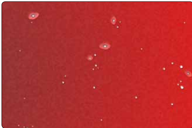
Figure 8-18. Example of fisheyes.
