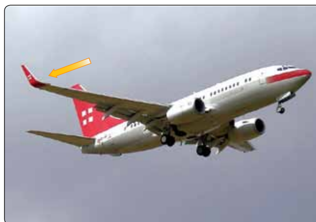
Figure 1-77. A winglet reduces aerodynamic drag caused by air spilling off of the wing tip.
