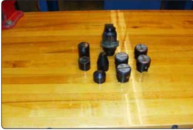
Figure 4-66. Shrinking and stretching tools.
