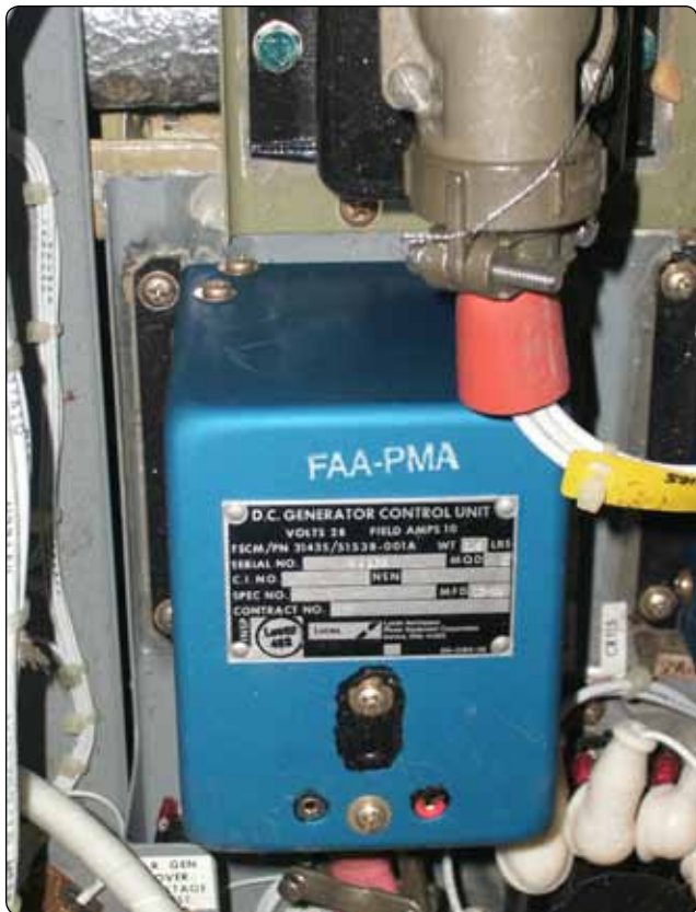
Figure 9-56. Generator control unit (GCU).
