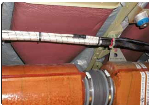
Figure 9-113. Shielded wire harness for flight control.
