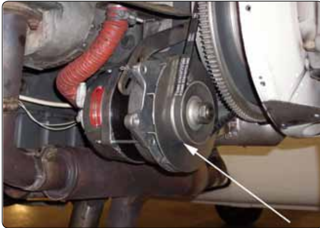
Figure 9-64. DC alternator installation.
