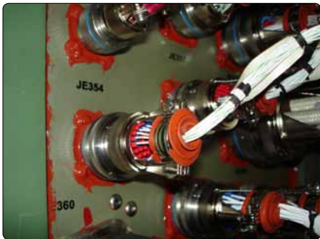
Figure 9-162. Backshells with strain relief.
