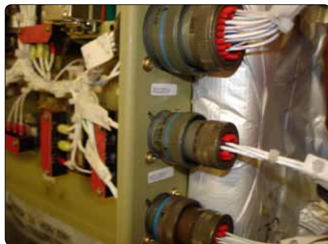
Figure 9-161. Connector arrangement to avoid wrong connection.
