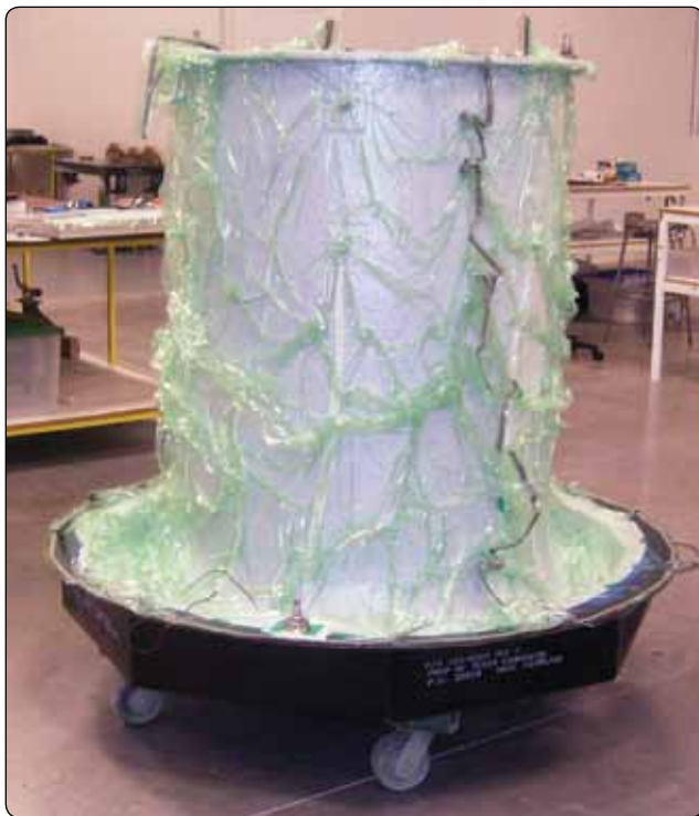
Figure 7-36. Bagging of complex part.
