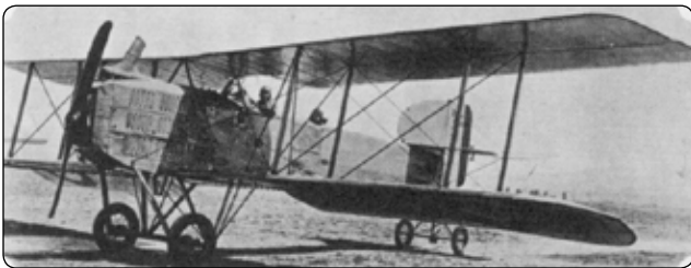
Figure 1-7. World War I aircraft were typically stacked-wing fabric-covered aircraft like this Breguet 14 (circa 1917).
