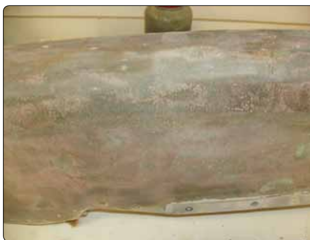
Figure 7-8. Copper mesh lightning protection material.
