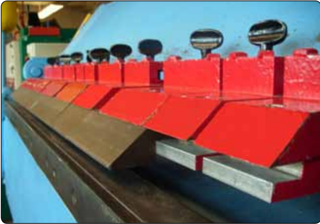
Figure 4-136. Brake radius nosepiece adjustment.
