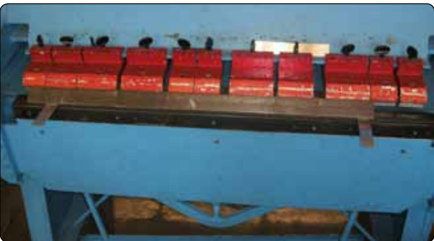
Figure 4-143. Brake alignment with two test strips 3-inches from each end.
