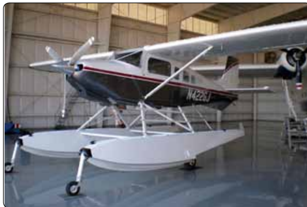
Figure 1-85. Retractable wheels make this aircraft amphibious.
