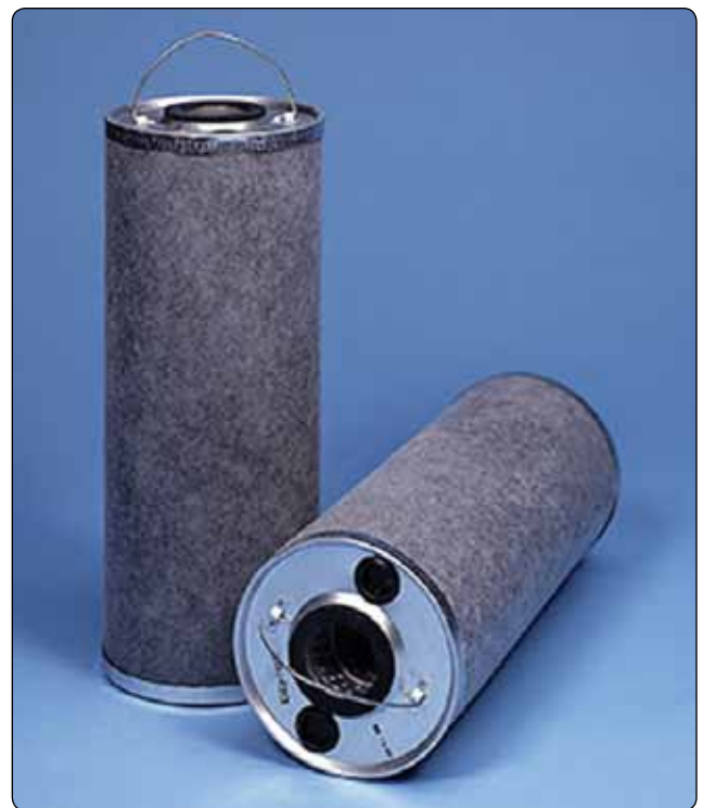
Figure 14-96. Clay filter elements remove surfactants. They are used in the fuel dispensing system before fuel enters the aircraft.
