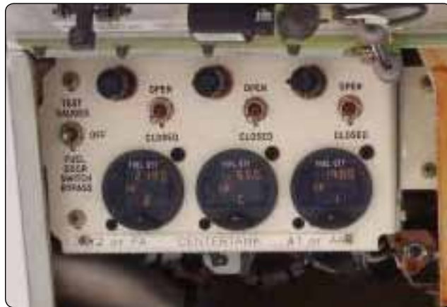
Figure 14-107. This panel at the pressure refueling station has valve position switches and quantity gauges to be used during refueling. Valve open position lights are adjacent to the switches for each tank.
