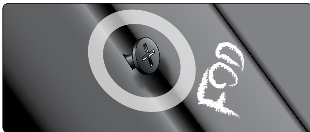
Figure 13-137. Marking of damaged area to enable closer inspection.
