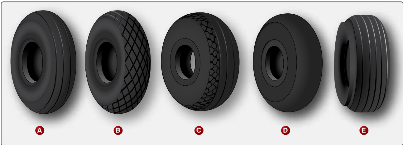
Figure 13-131. Aircraft tire treads are designed for different uses. A is a rib tread designed for use on paved surfaces. It is the most common aircraft tire tread design. B is a diamond tread designed for unpaved runways. C is an all weather tread that combines a ribbed center tread with a diamond tread pattern of the edges. D is a smooth tread tire found on older, slow aircraft without brakes designed for stopping. E is a chine tire used on the nose gear of aircraft with fuselage mounted jet engines to deflect runway water away from the engine intake(s).
