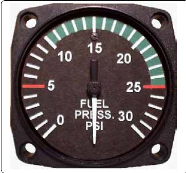
Figure 10-17. A typical analog fuel pressure gauge.
