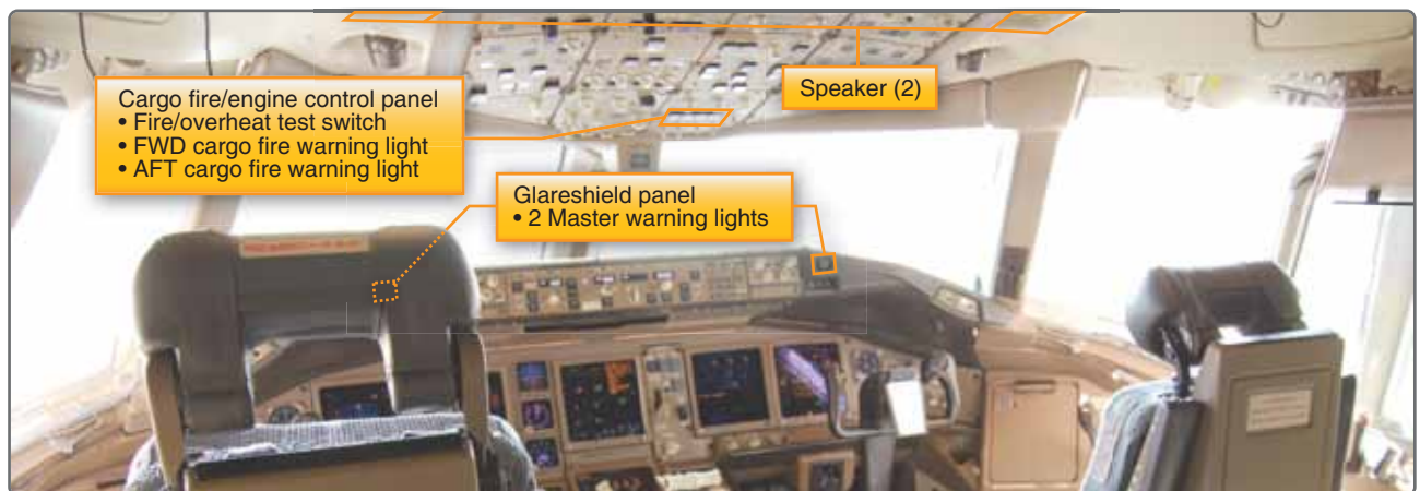
Figure 17-18. Cargo fire detection warning.
