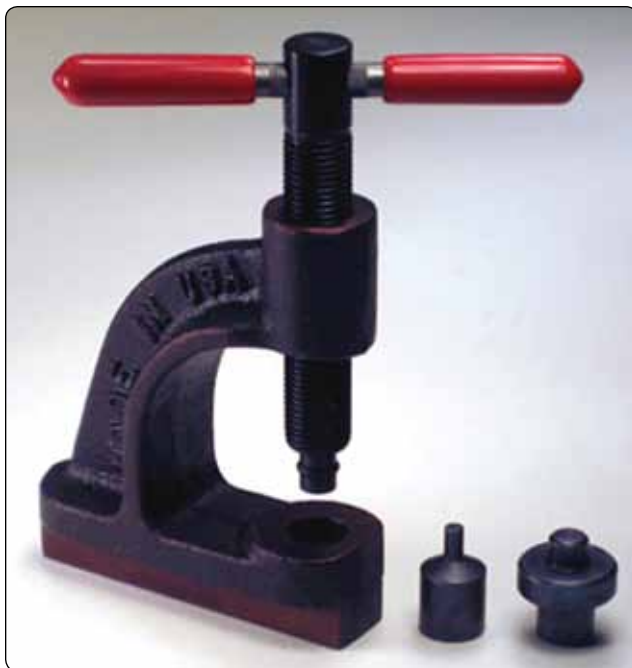
Figure 13-124. Rivet setting tool is used to install brake linings on Cleveland brake pressure plates and back plates.
