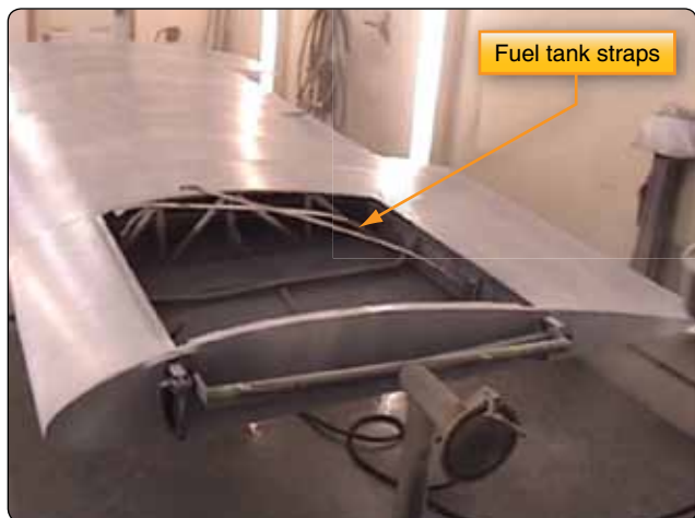
Figure 14-29. A fuel tank bay in the root of a light aircraft wing on a stand in a paint booth. Padded straps hold the fuel tank securely in the structure.
