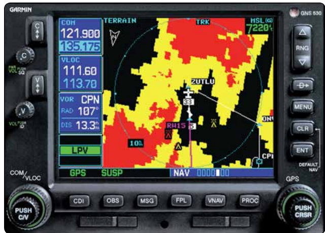
Figure 11-153. A GPS unit integrated with NAV/COM circuitry.
