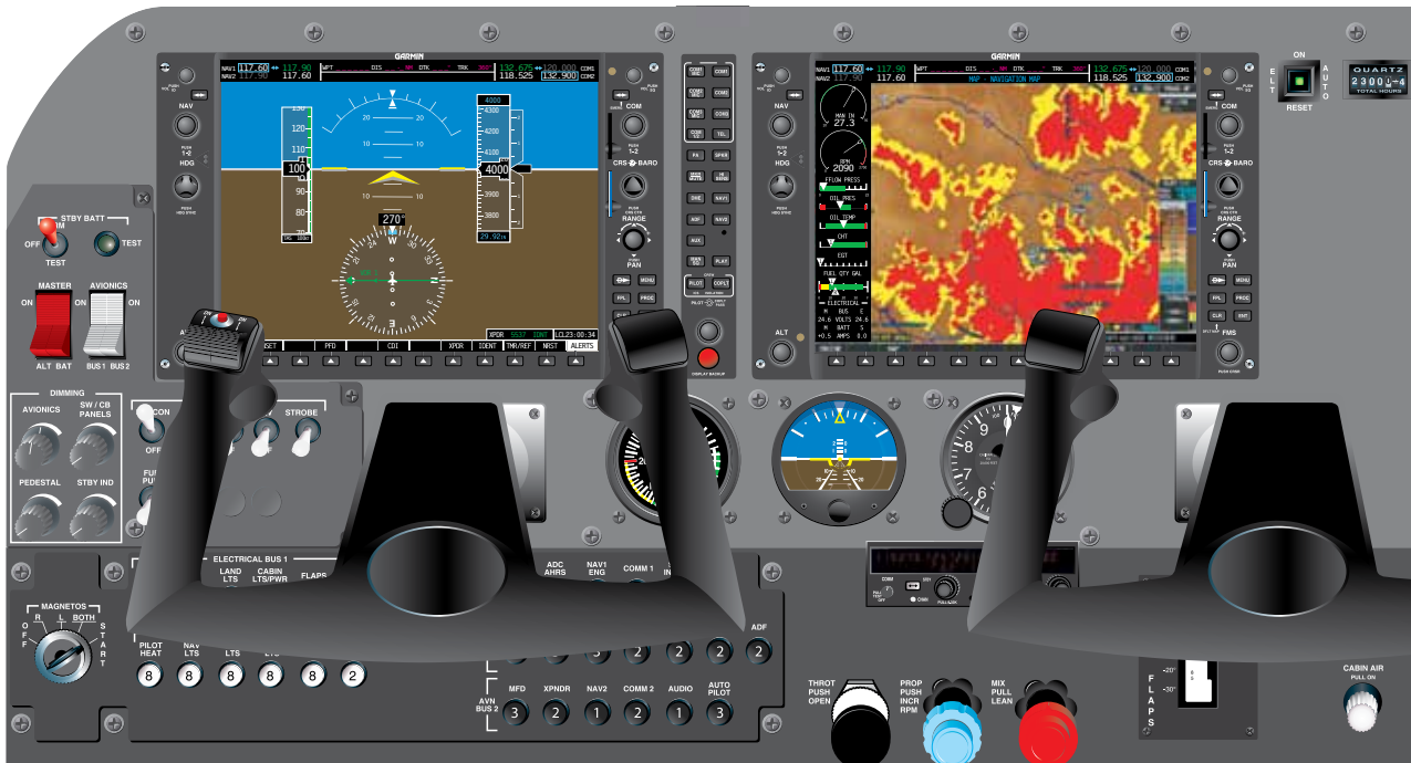
Figure 10-99. Instrumentation displayed within a glass cockpit using an attitude heading and reference system (AHRS) computer.
