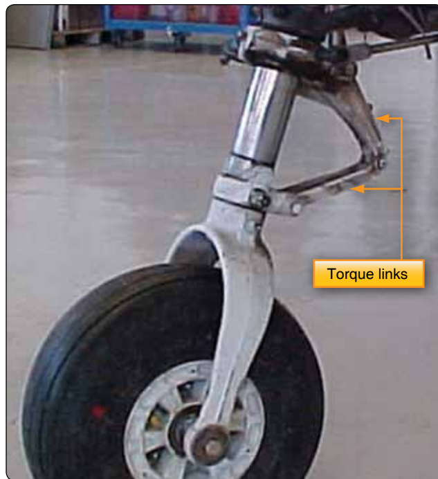
Figure 13-19. Torque links align the landing gear and retain the piston in the upper cylinder when the strut is extended.
