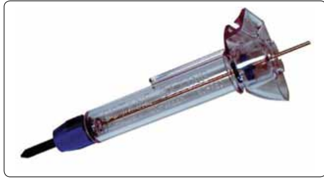
Figure 14-94. A sump drain tool used to open and collect fuel and contaminants from the fuel system sumps. Daily sump draining is part of the procedures needed to remove water from fuel that is to be delivered to the engine(s).
