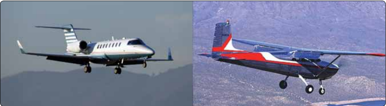
Figure 13-6. Tricycle-type landing gear with dual main wheels on a Learjet (left) and a Cessna 172, also with tricycle gear (right).
