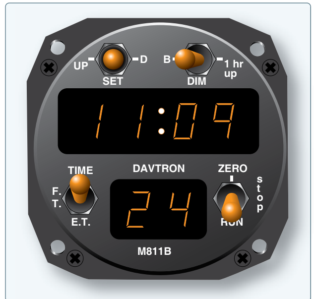
Figure 10-132. A typical aircraft electronic clock.
