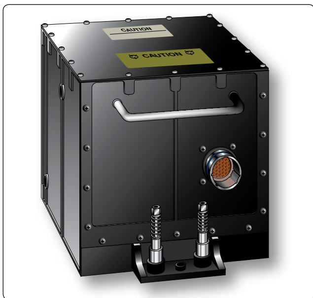
Figure 11-156. A modern micro-IRS with built-in GPS.
