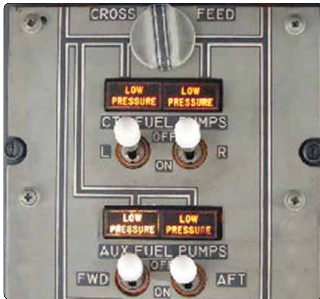
Figure 14-88. A transport category aircraft fuel panel with low pressure warning lights for each fuel boost pump.
