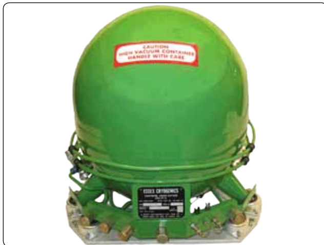
Figure 16-6. A spherical liquid oxygen onboard container used by the military.
