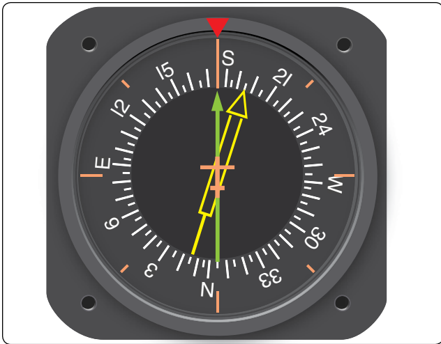
Figure 10-85. A radio magnetic indicator (RMI) combines a slaved gyro heading indication (red triangle at top of gauge) with magnetic bearing information to a VOR station (solid pointer) and an ADF station (hollow pointer).
