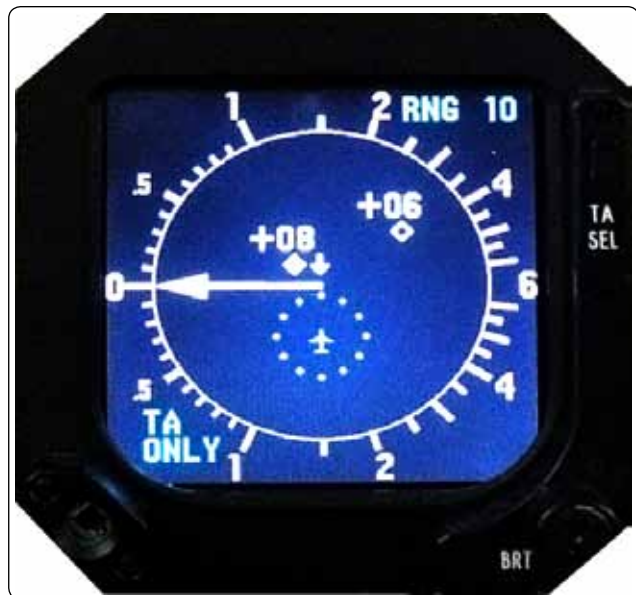
Figure 11-132. TCAS information displayed on an electronic vertical speed indicator.
