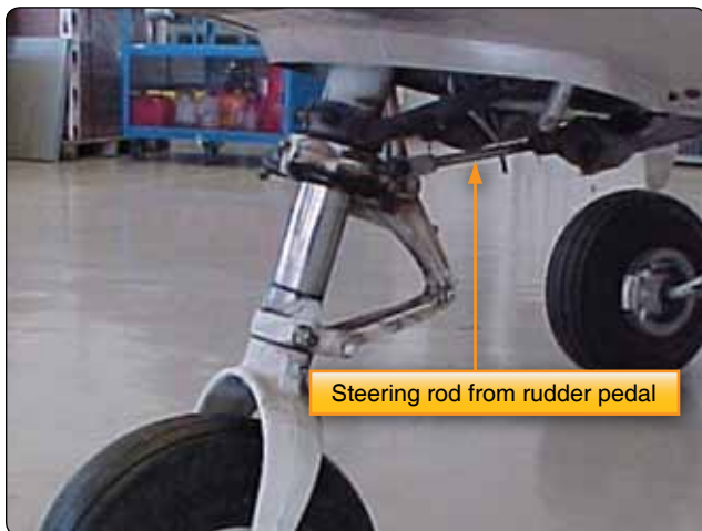
Figure 13-50. Nose wheel steering on a light aircraft often uses a push-pull rod system connected to the rudder pedals.
