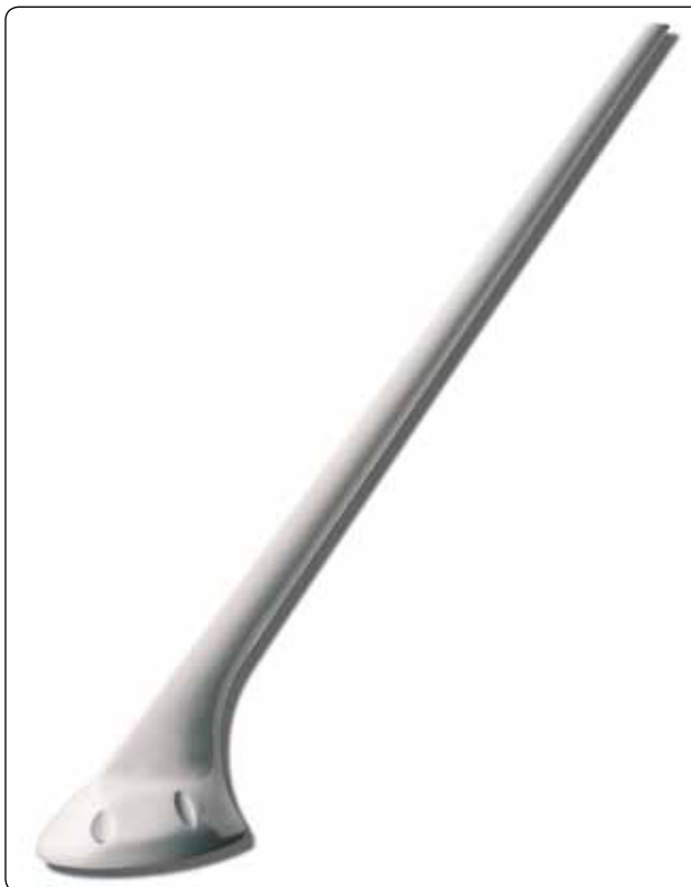
Figure 11-90. Many antenna are canted for better reception.
