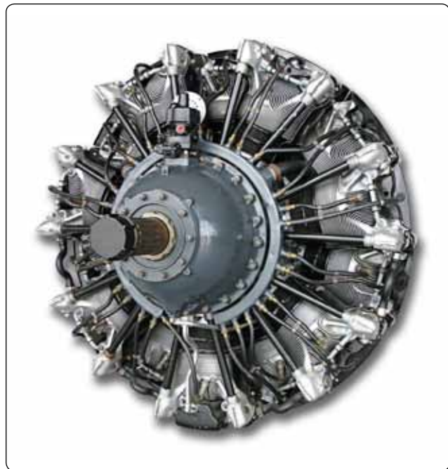
Figure 16-43. The radial engine supercharger cannot be used since fuel is introduced before the supercharger impeller compresses the air.
