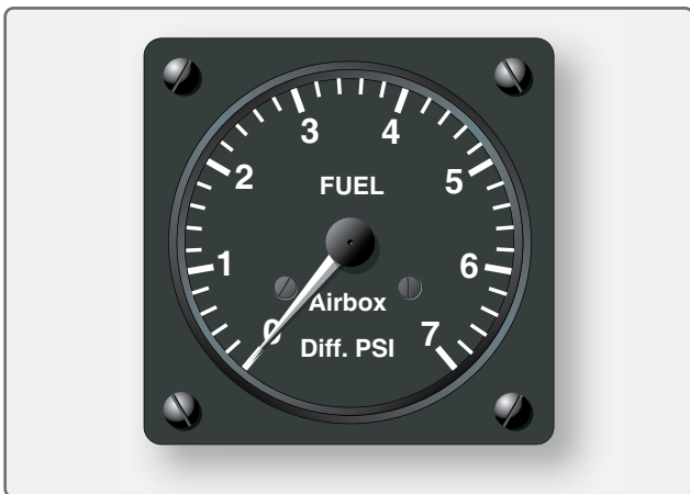
Figure 14-85. A differential fuel pressure gauge used on complex and high-performance reciprocating-engine aircraft compares the fuel inlet pressure to the air inlet pressure at the fuel metering device.
