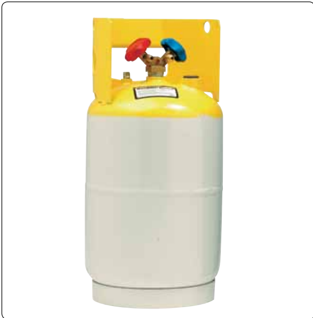
Figure 16-89. A 30 pound R134a refrigerant container with dual fittings. The fitting controlled by the blue valve wheel opens to the vapor space above the liquid refrigerant for connection to the low side of the vapor cycle system. The fitting controlled by the red valve wheel draws liquid refrigerant from the bottom of the cylinder through a stand tube. This fitting is connected to the system high side. On containers without dual fittings, the container must be inverted to deliver liquid refrigerant through a connected hose.
