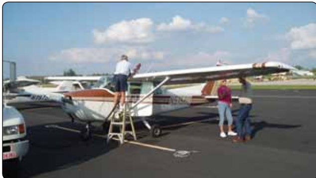
Figure 14-106. Over-the-wing refueling a Cessna.
