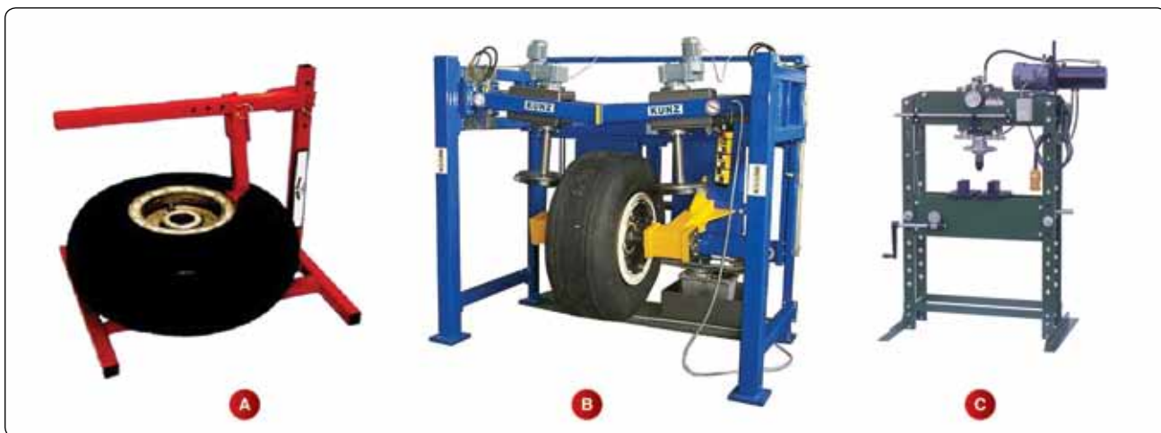
Figure 13-63. Tire beads must be broken from the wheel to remove the tire. A mechanical removal tool designed for breaking the bead is shown in (A); a hydraulic press designed with the capacity for large aircraft wheels is shown in (B); and an arbor press is shown in (C). All are tools available to the technician for this purpose.
