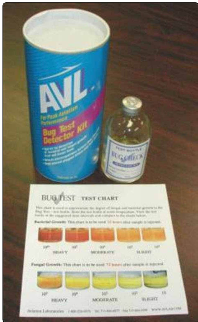
Figure 14-101. Fuel bug test kits identify the level of bacteria and fungus present in a fuel load by comparing the color of a treated sample with a color chart.
