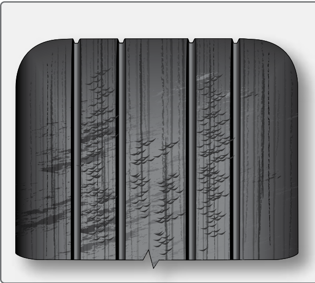
Figure 13-142. Chevron cuts in a tire are caused by operation on grooved runway surfaces. Shallow chevron cuts are permitted on aircraft tires.
