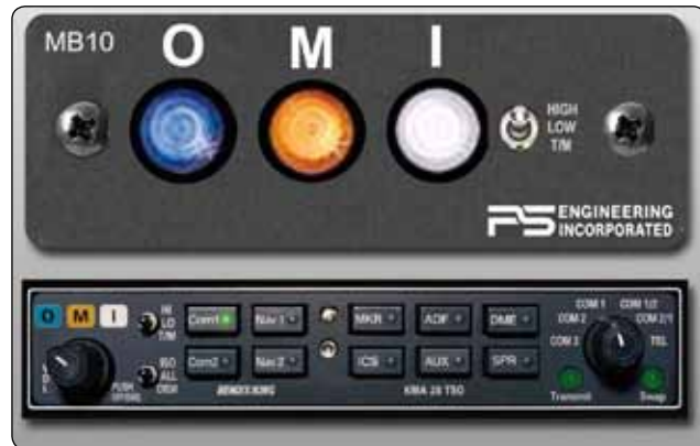
Figure 11-116. Various marker beacon instrument panel display lights.
