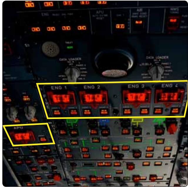
Figure 17-16. Engine and APU fire switches on the cockpit center overhead panel.
