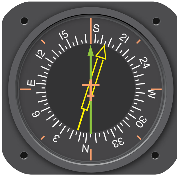
Figure 11-109. A radio magnetic indicator (RMI) combines a magnetic compass, VOR, and ADF indications.
