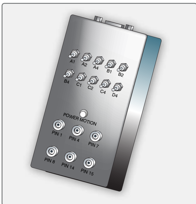
Figure 11-129. A handheld transponder test unit.
