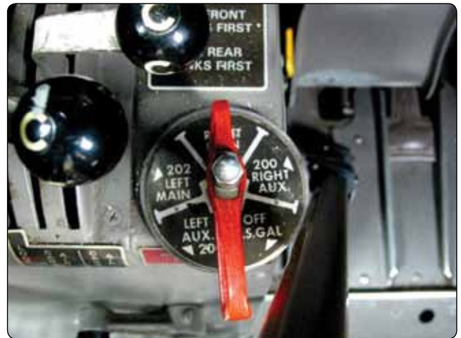
Figure 14-39. Detents for each position, an indicating handle, and labeling aid the pilot in knowing the position of the fuel valve.
