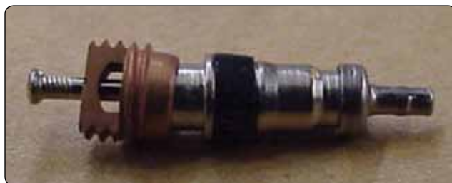
Figure 13-148. The tire valve core should be removed after the tire is completely deflated and before the tire and wheel assembly is removed from the aircraft.
