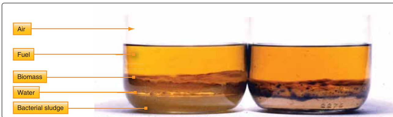
Figure 14-97. This fuel-water sample has microbial growth at the interface of the two liquids.
