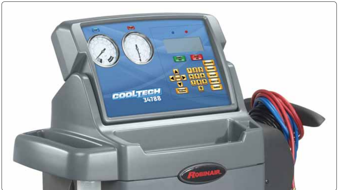
Figure 16-88. A modern refrigerant recovery/charge/recycle service unit. Electronic control of solenoid activated valves combine with a built-in system for recovering, recycling, and recharging. A built-in vacuum pump and heated refrigerant reservoir are also included.
