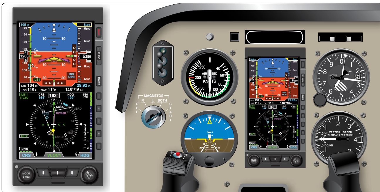
Figure 11-71. A retrofit digital data display.
