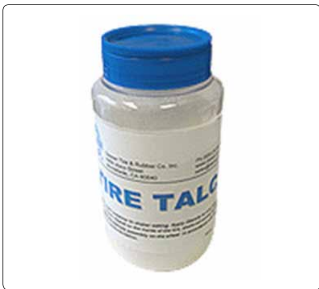
Figure 13-155. Tire talc is used on the inside of tube-type tires and the outside of aircraft tubes. This prevents binding and allows the tube to expand without stress into place within the tire.
