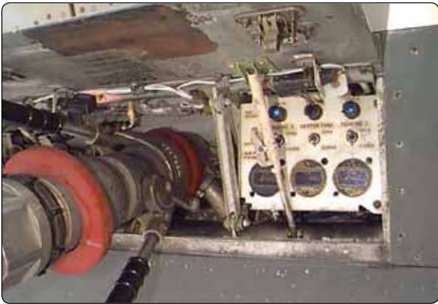
Figure 14-22. A central pressure refueling station on a transport category aircraft allows all fuel tanks to be filled from one position.
