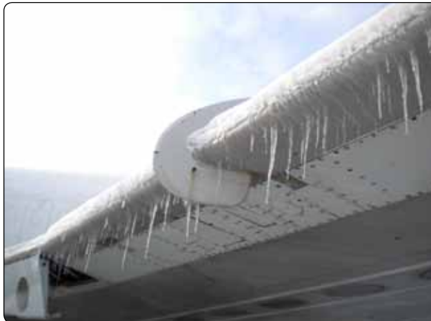
Figure 15-1. Formation of ice on aircraft leading edge.
