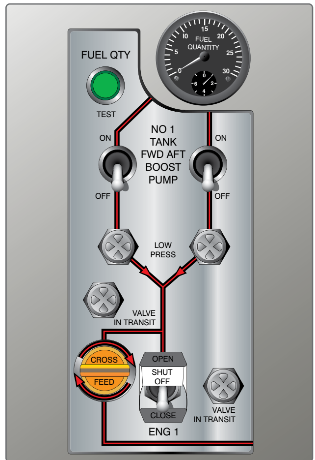
Figure 14-89. Valve-in-transit lights are used on this section of a transport category aircraft fuel panel. Low boost pump pressure lights that look the same are also on the panel.
