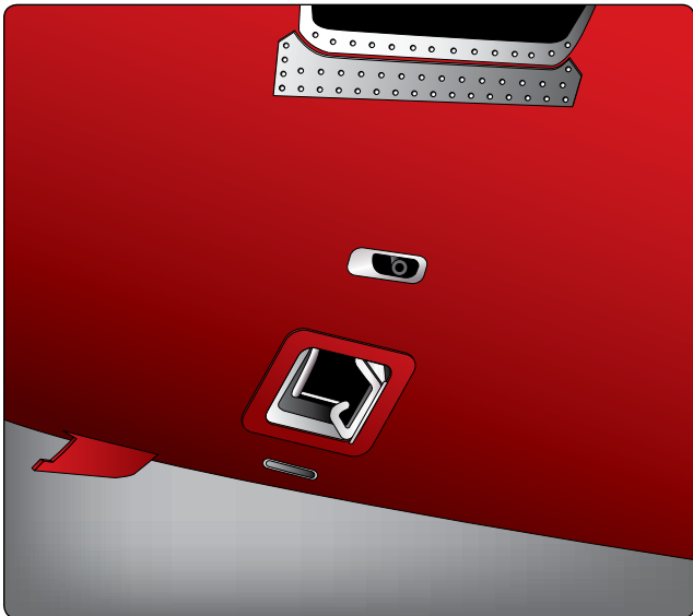
Figure 16-55. This outflow valve on a transport category aircraft is normally operated by an ac motor controlled by a pressure controller in the electronics equipment bay. A second ac motor on the valve is use when in standby mode. A dc motor also on the valve is used for manual operation.
