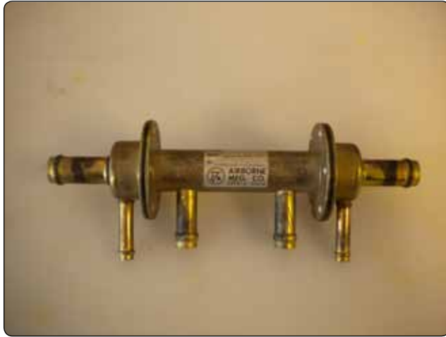
Figure 15-28. A manifold assembly used in multiengine aircraft deice systems.
