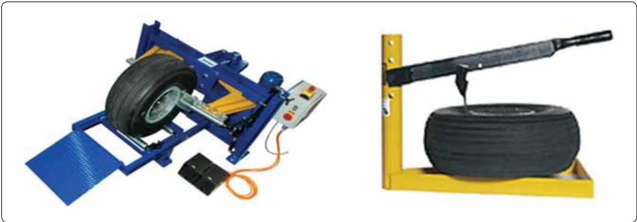
Figure 13-150. An electrohydraulic tire bead breaker (left) used on large tires and a manual tire bead breaker (right) used on small tires.
