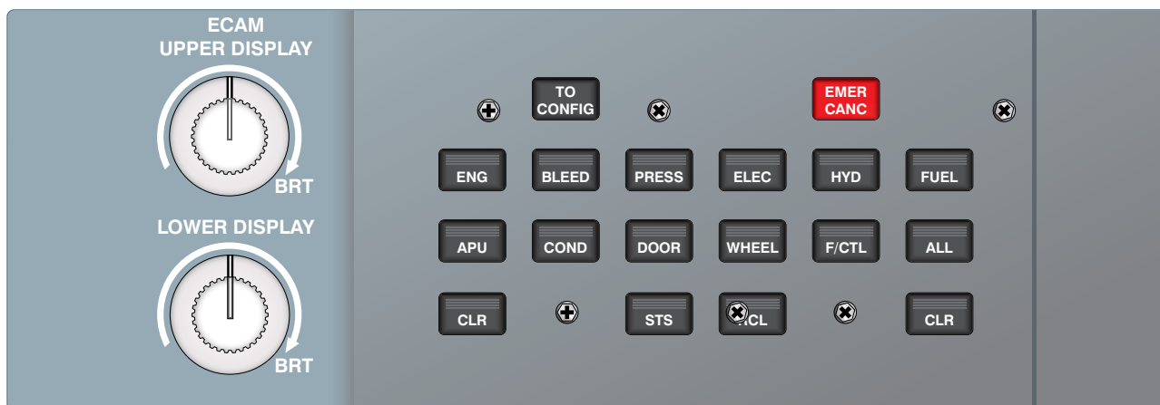
Figure 10-121. An ECAM display control panel.
