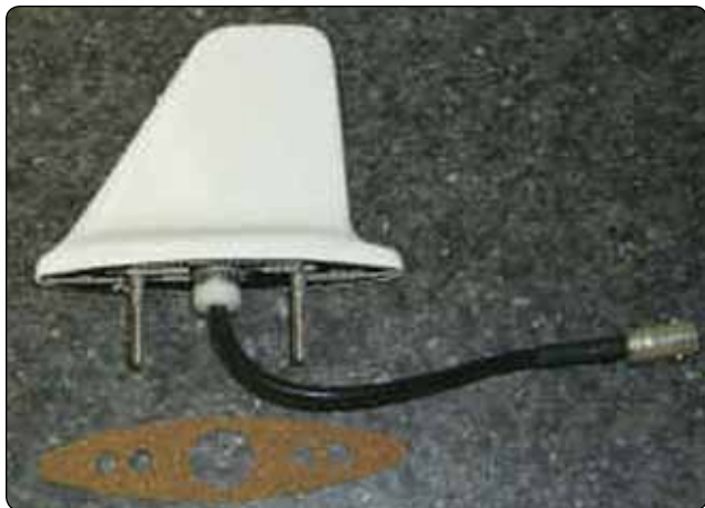
Figure 11-121. A typical aircraft mounted DME antenna.
