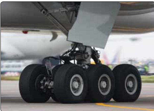
Figure 13-9. Triple bogie main landing gear assembly on a Boeing 777.
