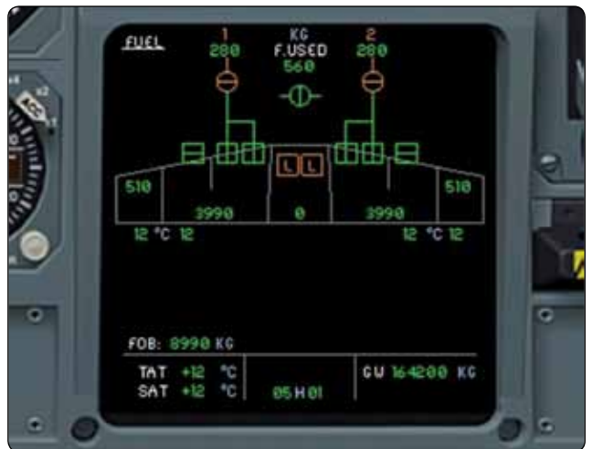
Figure 14-40. The graphic depiction of the fuel system on this electronic centralized aircraft monitor (ECAM) fuel page includes valve position information.
