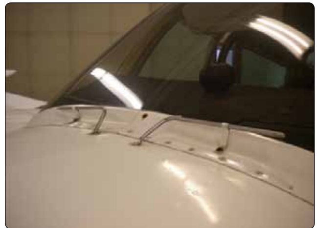
Figure 15-46. Chemical deicing spray tubes.
