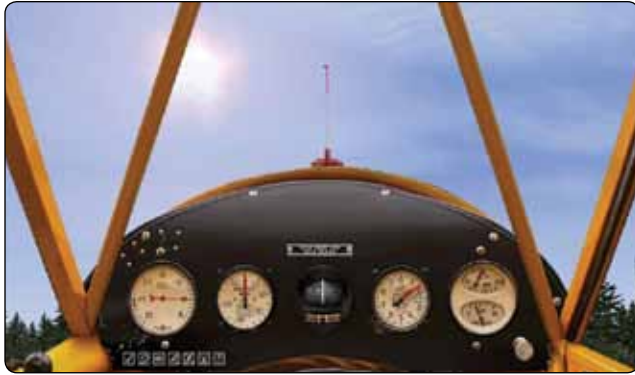
Figure 14-67. The fuel quantity indicator on this Piper Cub is a float attached to a rod that protrudes through the fuel cap.
