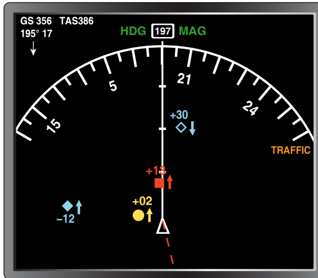
Figure 11-133. TCAS information displayed on a multifunction display. An open diamond indicates a target; a solid diamond represents a target that is within 6 nautical miles of 1,200 feet vertically. A yellow circle represents a target that generates a TA (25-48 seconds before contact). A red square indicates a target that generates an RA in TCAS II (contact within 35 seconds). A (+) indicates the target aircraft is above and a (-) indicates it is below. The arrows show if the target is climbing or descending.
