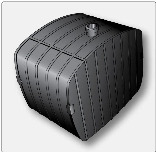
Figure 14-30. A fuselage tank for a light aircraft.
