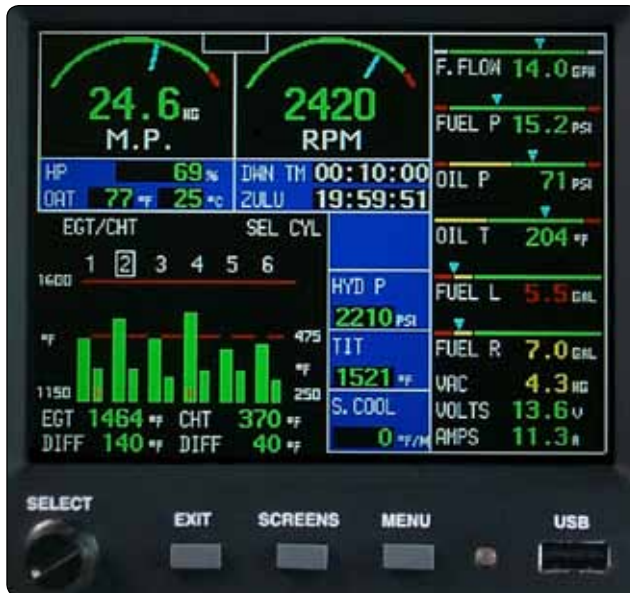
Figure 11-72. A digital data display dedicated to the depiction of engine and airframe system parameter status.
