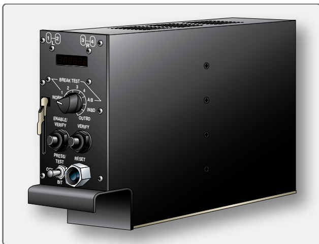
Figure 13-108. A rack mounted antiskid control unit from an airliner.
