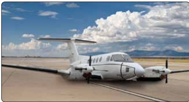
Figure 14-3. Aircraft fuel tanks must be designed to retain fuel in the event of a gear-up landing. The fuel system drain valve should be located to prevent spillage.
