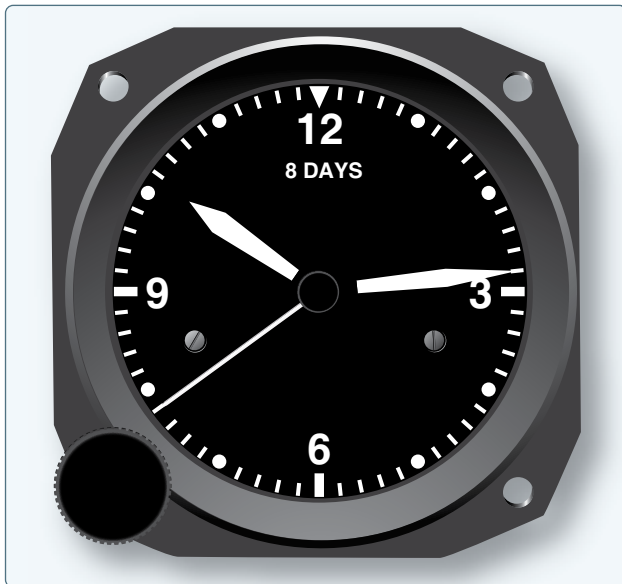
Figure 10-131. A typical mechanical 8-day aircraft clock.
