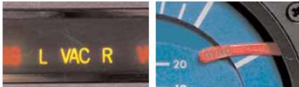
Annunciators and flags provide an early indication of a pneumatic system failure.
